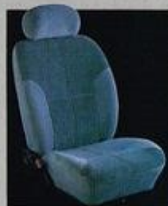
The reclining front seats have padded, fully adjustable head restraints, and the occurrence of seat frame-recessed anti-lift brackets.
